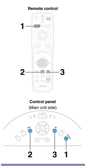
A picture may be expanded on the upper side if projected upward from the projector lifted up by the foot adjuster. The projector can correct this keystone distortion.
